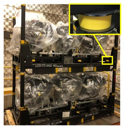
This was a major win for the OEM, helping to eliminate part damage in the field. The solution was derived over a few short weeks and would allow the OEM to meet it's launch requirements. These vibration dampening pucks are now used worldwide.
